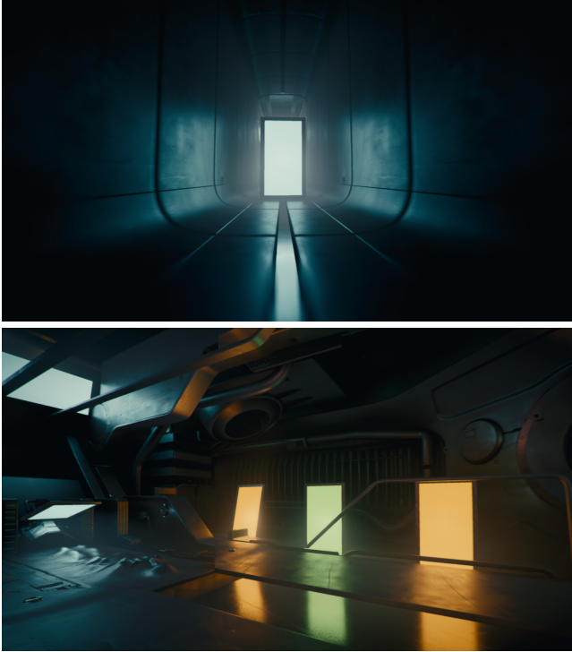
Figure 8: Integration into a game engine. The scene contains 8 rectangular lights and the total rendering time per frame is 15ms on an NVIDIA GeForce GTX 980 GPU at 1280 \times 720 pixels.
